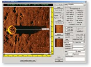
Sonar contacts and all of their measurements and attributes are stored in a relational database to allow unlimited report generation options. Use the Contact Report Generator to search on any data field, such as all contacts with a height greater than 3.0 meters. The results might include the cable spool shown in the image at left that otherwise would be very hard to pinpoint as an object of interest.
