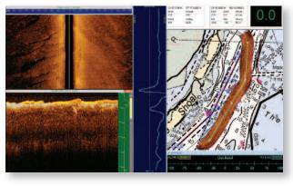
Flexible viewing options in SonarWiz 5 enable you to see simultaneously what each of several devices is capturing during the survey mission. This example shows the results of sidescan (upper left), sub-bottom (lower left), magnetometer (center), along with your route overlaid onto the appropriate chart (right).
